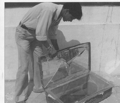
Sunny prepares lunch; Manoj then cooks it on the roof in an upcycled solar cooker made from a rusted trunk, broken mirror, rubber tire tubes, and an old car windshield.
